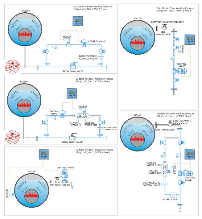
The customised prefabricated piping assemblies are provided with IBR certification. With our certified team, we can undertake site installation.
